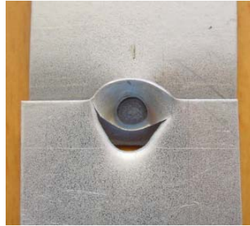
Figure 5: Failure mode in tensile test of TRIP700 resistance spot weld.
