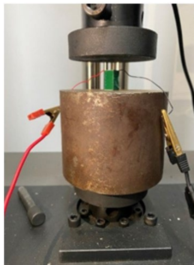
Figure 4 Detailed diagram of zero displacement test of piezoelectric ceramic actuator
