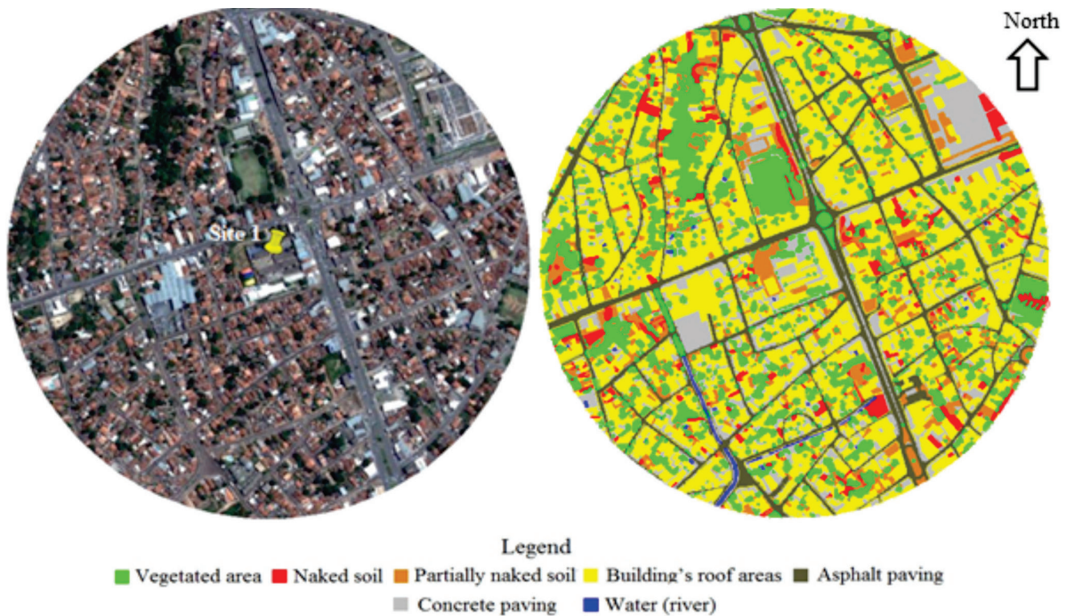
Figure 2 – Land use and land occupation inside the circle of influence for site 1 (radius of 500m).
