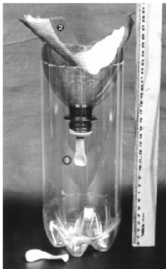
Recycled 2 liter plastic bottle for larvae isolation (Baermann method). Note the small latex baloon (1) occluding the funnel or resting next to the bottle and the plastic mesh (2) holding the gauze.
