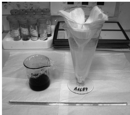
Fig. 1: conical glass jar used for Lutz's sedimentation technique.
