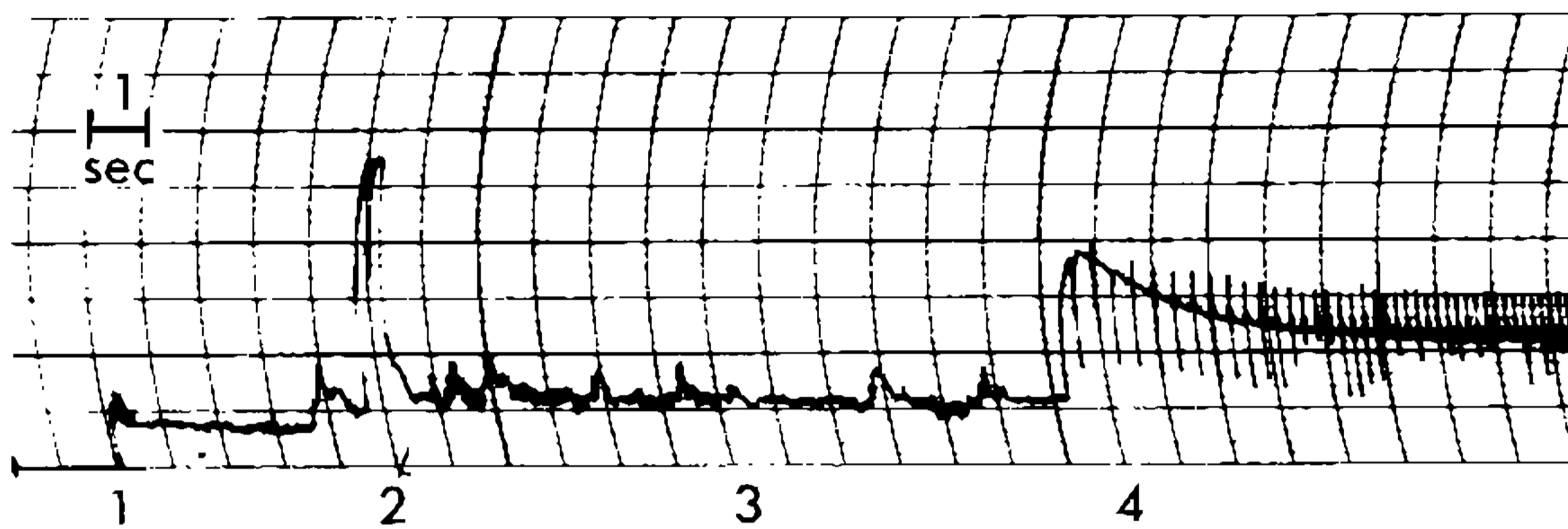
Fig. 2: Typical record of electrical activity associated with R. prolixus feeding on saline and ATP, and using apparatus shown in Fig. 1. Vertical axis represents voltage at preamplifier input (arbitrary units). 1. Initial penetration. 2. "Sampling" – opening of functional mouth with one pump stroke (negative-going "spike"); 3. Maxillary probing, with somewhat irregular 1-3 second periodicity correlated with protraction-retraction cycles; 4. Start of pumping phase, with individual pump strokes showing increase in pump frequency from 2\text{ s}^{-1} to 6\text{ s}^{-1} . Modified from Smith & Friend, 1970.
