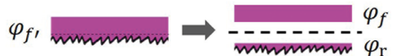
Figure 3. The one-side-rough film f' can be decomposed, in terms of power dissipation and energy stored, into the smooth film f and the rough interface r .
