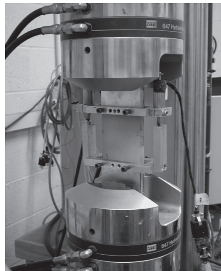
Figure 5. Uniaxial tensile test setup.
