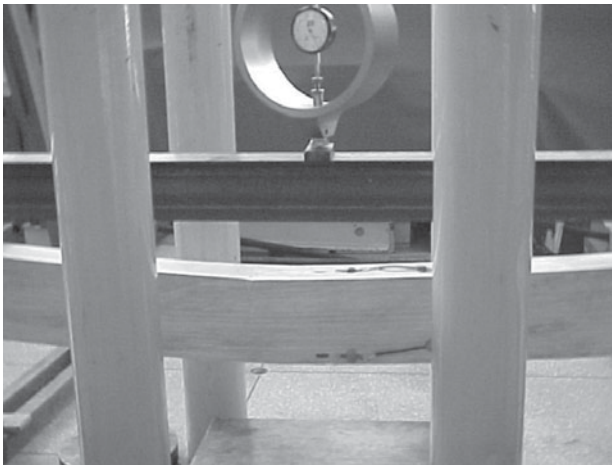
Figure 11. Deflection, followed by tensile failure of the beam.
