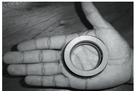
Figure 3. Toroidal core assembled with nanocrystalline alloy with rectangular cross-section.
