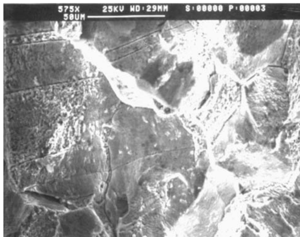
Figure 10. Scanning electron micrographs for 254 SMO sensitized, after SSRT in 5 mol/L H 2 SO 4 / 1 mol/L NaCl solution at 25 °C.
