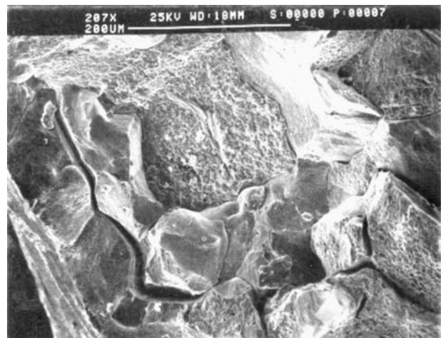
Figure 12. Scanning electron micrographs for sensitized UNS S10276, after SSRT in 2.9 mol/L NaCl / 0.1 mol/L HCl at 80 °C.
