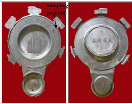
Figure 2. Physical drawing and sampling position of thin-walled diecasting part.
