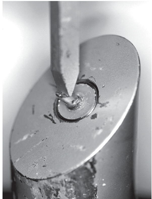
Figure 8. Application of the load ( F < PLL ) in a Ag specimen.
