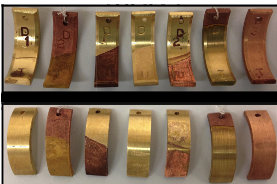
Figure 2. Front (top) and back (bottom) images of brass samples 1 through 7 (left to right) after corrosion testing in ammonia solutions and cleaning in 1M sulphuric acid pickling solution.
