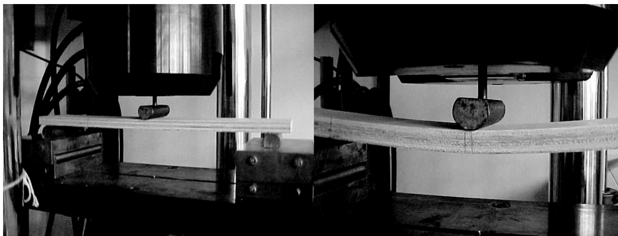
Figure 2. Mechanical test for determination of static bending properties.
