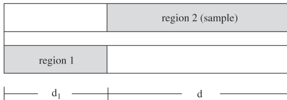
Figure 1. Sketch of the coaxial line structure. Region 2 with length d (longitudinal section) contains the dielectric sample under investigation. Region 1 contains a dielectric material with lower permittivity and loss.
