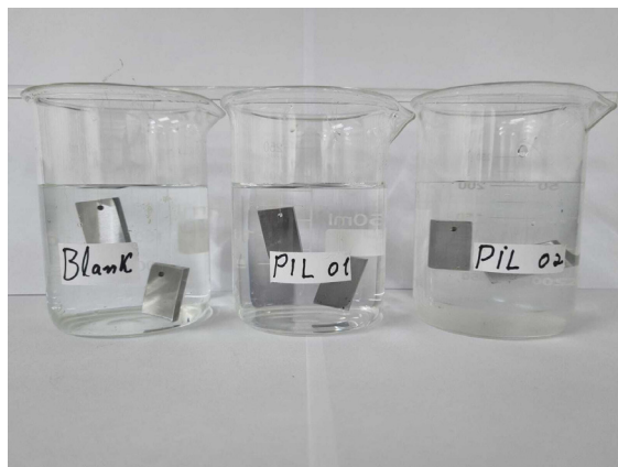
Figure 4. Corrosion test samples immersed in solution (3.5% wt. NaCl) for the weight loss test with pH variation.
