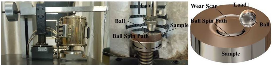
Figure 3. MGG-02 high temperature reciprocating friction and wear testing machine: (a) experimental setup and (b) working principle
