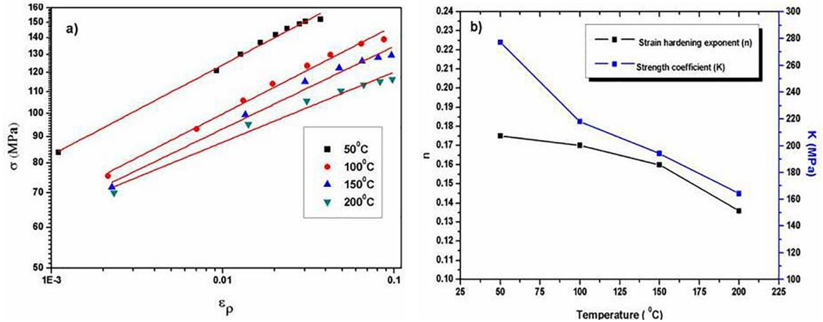
Figure 6. (a) log-log plot of  $\sigma$  vs.  $\epsilon_p$  (b) variation of  $n$  and  $K$  with temperature.
