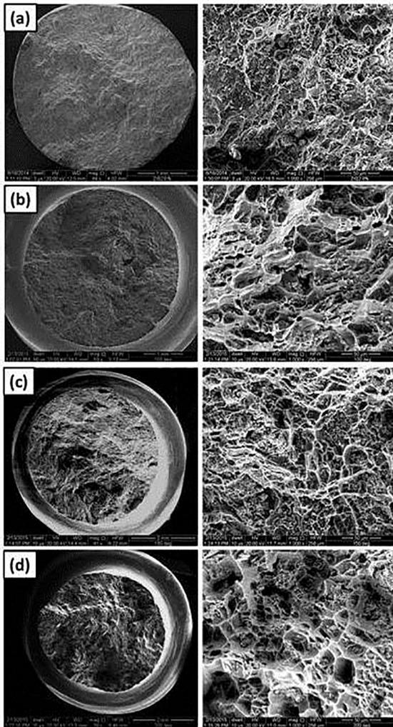
Figure 7. Fractographs of composite with 9 vol. %  $ZrB_2$  at different temperatures (a) RT (b) 100°C (c) 150°C and (d) 200°C.
