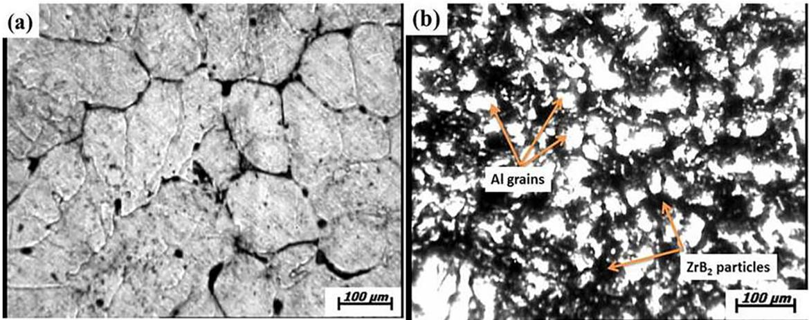
Figure 3. Optical micrograph of (a) alloy with 0 vol. %  $ZrB_2$  (b) composite with 9 vol. %  $ZrB_2$ .
