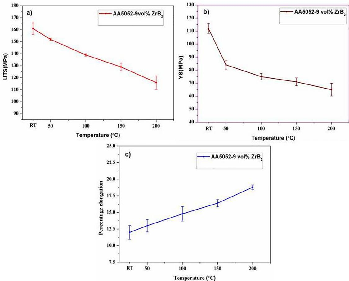
Figure 5. Variation of (a) UTS (b) YS and (c) percentage elongation with temperature.
