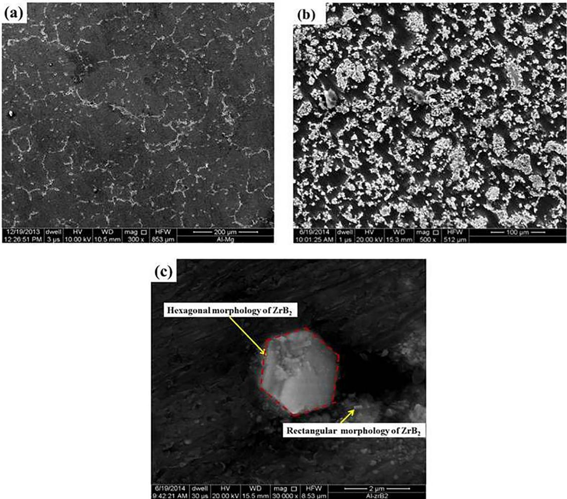
Figure 4. SEM micrograph of (a) alloy with 0 vol. %  $ZrB_2$  (b) composite with 9 vol. %  $ZrB_2$  (c)  $ZrB_2$  morphology at high magnification.
