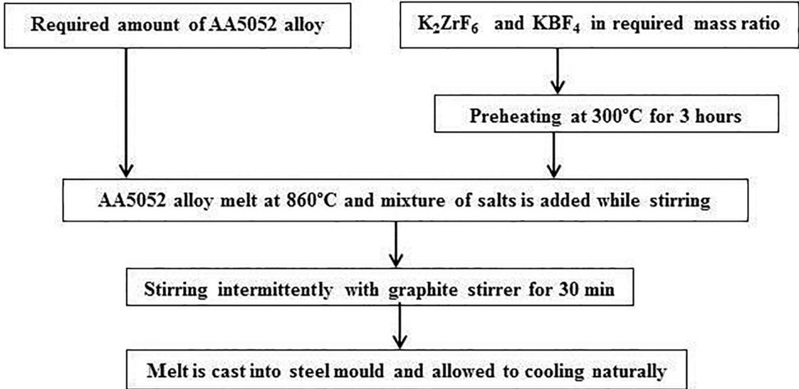
Figure 1. Flow chart for synthesizing the composite.
