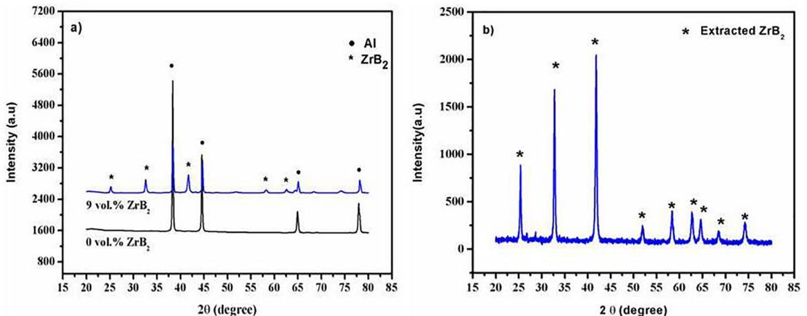
Figure 2. XRD pattern of (a) 0 and 9 vol. % ZrB<sub>2</sub> composite (b) extracted particle of ZrB<sub>2</sub>.
