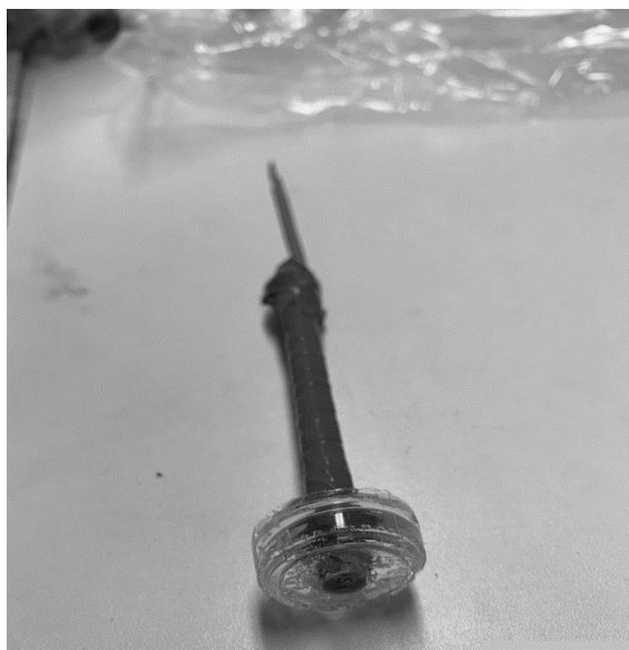
Figure 1. Steel bar after pre-treatment and preparation with epoxy resin.
