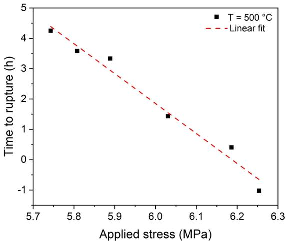
Figure 4. Dependence of time to rupture (h) on applied stress (MPa)<sup>3,6</sup>.
