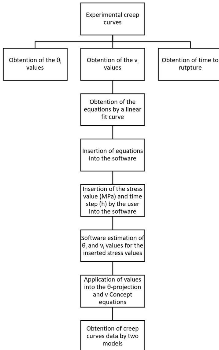
**Figure 2.** Flowchart describing the steps performed to predict creep curves following the  $\theta$ -projection and  $\nu$  Concept methodologies.
