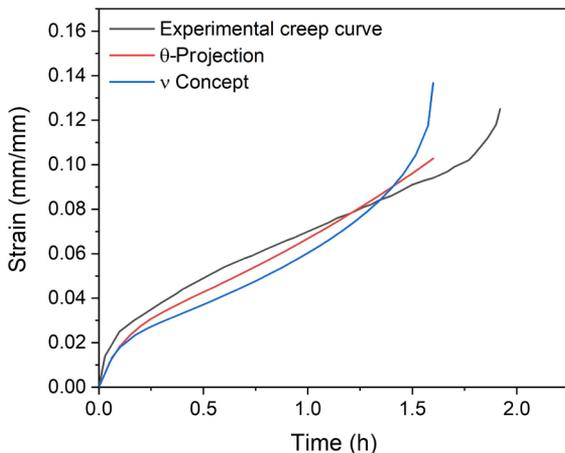
Figure 5. Creep curves calculated by Equations 1 and 2 and experimental data at 465 MPa.
