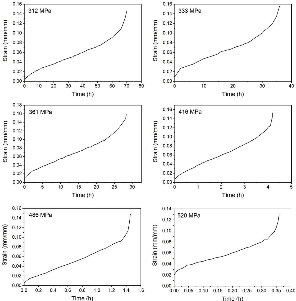
**Figure 1.** Ti-6Al-4V experimental creep curves (312 to 520 MPa) at 500 °C used to determine the  $\theta$  and  $\nu$  parameters<sup>3,6</sup>.
