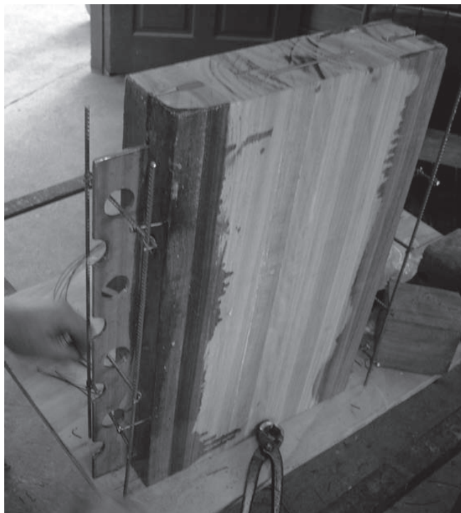
Figure 7. Specimens type SP-III being constructed.
