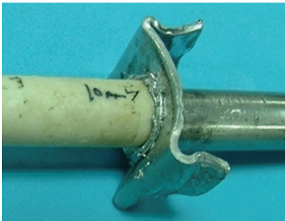
Figure 12. Appearance of friction welded alumina-mild steel with aluminum alloy interlayer.
