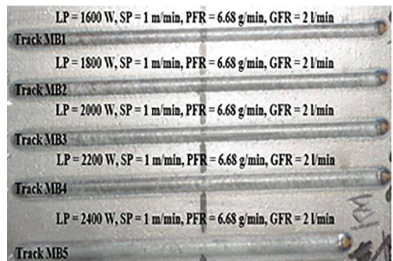
Figure 2. Physical appearance of the Ti6Al4V+B 4 C deposits with respect to laser power.
