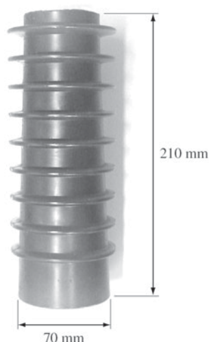
Figure 1. Insulator of the indoor type manufactured with polyurethane resin.
