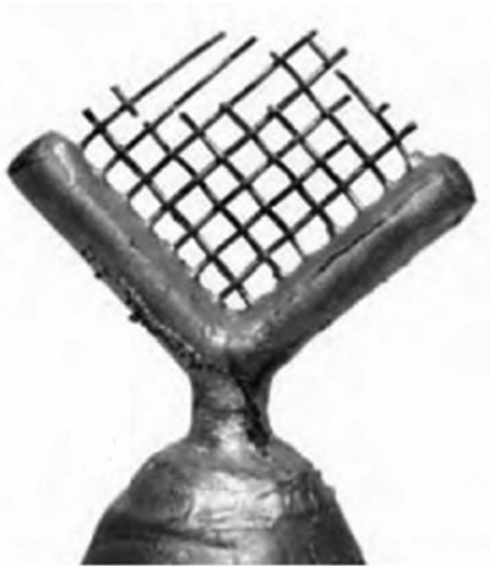
Figure 2. Casting for castability evaluation with incomplete cast segments.
