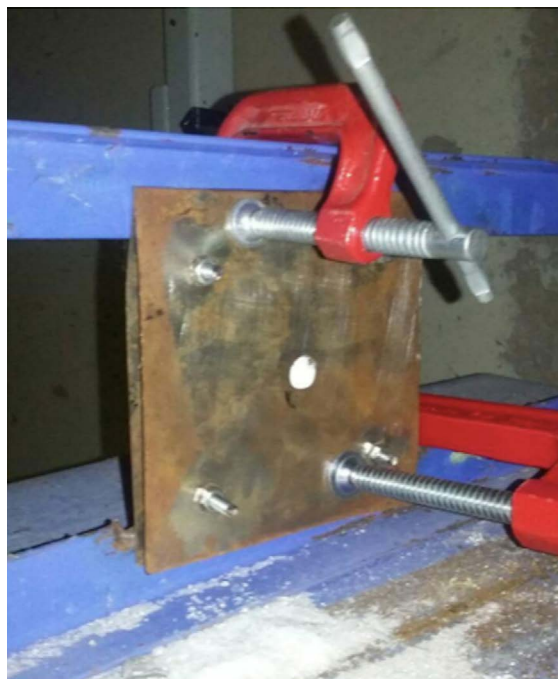
Figure 1. Fixing of samples confined by the steel plates for the ballistic tests.
