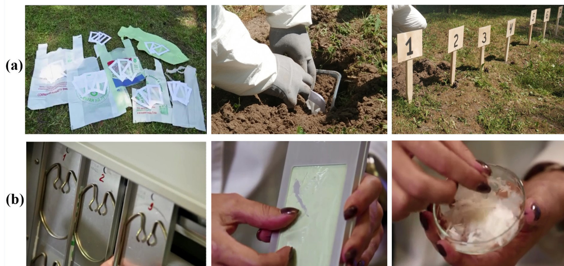
Figure 1. (a) The procedure of the soil test; (b) The stages of the accelerated weathering test (climatic chamber).
