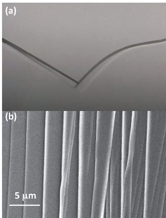
**Figure 3:** (a) outer surface and (b) SEM image obtained near the crease mark of the bent alloy ribbon  $\text{Fe}_{88}\text{Mo}_2\text{Si}_5\text{B}_5$  annealed at 823 K for 600 s.
