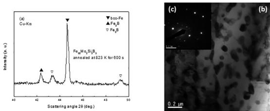
**Figure 6:** (a) High resolution XRD patterns (Cu-K $\alpha$ ) and (b) Bright-field image with corresponding (c) selected area electron diffraction pattern of  $\text{Fe}_{88}\text{Mo}_2\text{Si}_5\text{B}_5$  ribbon after annealing at 823 K for 600 s.
