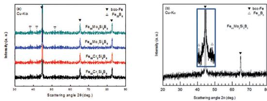
**Figure 1:** (a) X-ray diffraction pattern of  $\text{Fe}_{90-x}\text{Si}_5\text{B}_5\text{M}_x$  ( $\text{M}=\text{Cr}, \text{Mo}$ ;  $x=1, 2$ ) alloys with Cu-K $\alpha$  radiation. (b) high resolution scanned XRD patterns of  $\text{Fe}_{88}\text{Mo}_2\text{Si}_5\text{B}_5$  alloy.
