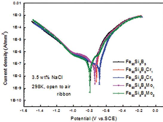
**Figure 5:** Polarization curves of the  $\text{Fe}_{90-x}\text{Si}_5\text{B}_5\text{M}_x$  ( $M = \text{Cr}$  or  $\text{Mo}$ ;  $x = 1, 2$ ) ribbon alloys in 3.5mass% NaCl solution at 298K. The ribbons were annealed at 823 K for 600s.
