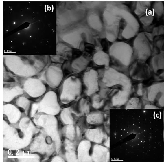
**Figure 2:** (a) Bright-field and (b) (c) selected area electron diffraction patterns in different phases of the  $\text{Fe}_{88}\text{Mo}_2\text{Si}_5\text{B}_5$  alloy.
