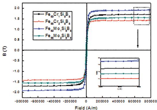
**Figure 4:**  $B$ - $H$  hysteresis loops of  $\text{Fe}_{90-x}\text{Si}_5\text{B}_5\text{M}_x$  ( $M=\text{Cr}, \text{Mo}; x=1, 2$ ) ribbon as-spun alloys under an applied field of 800 kA/m.
