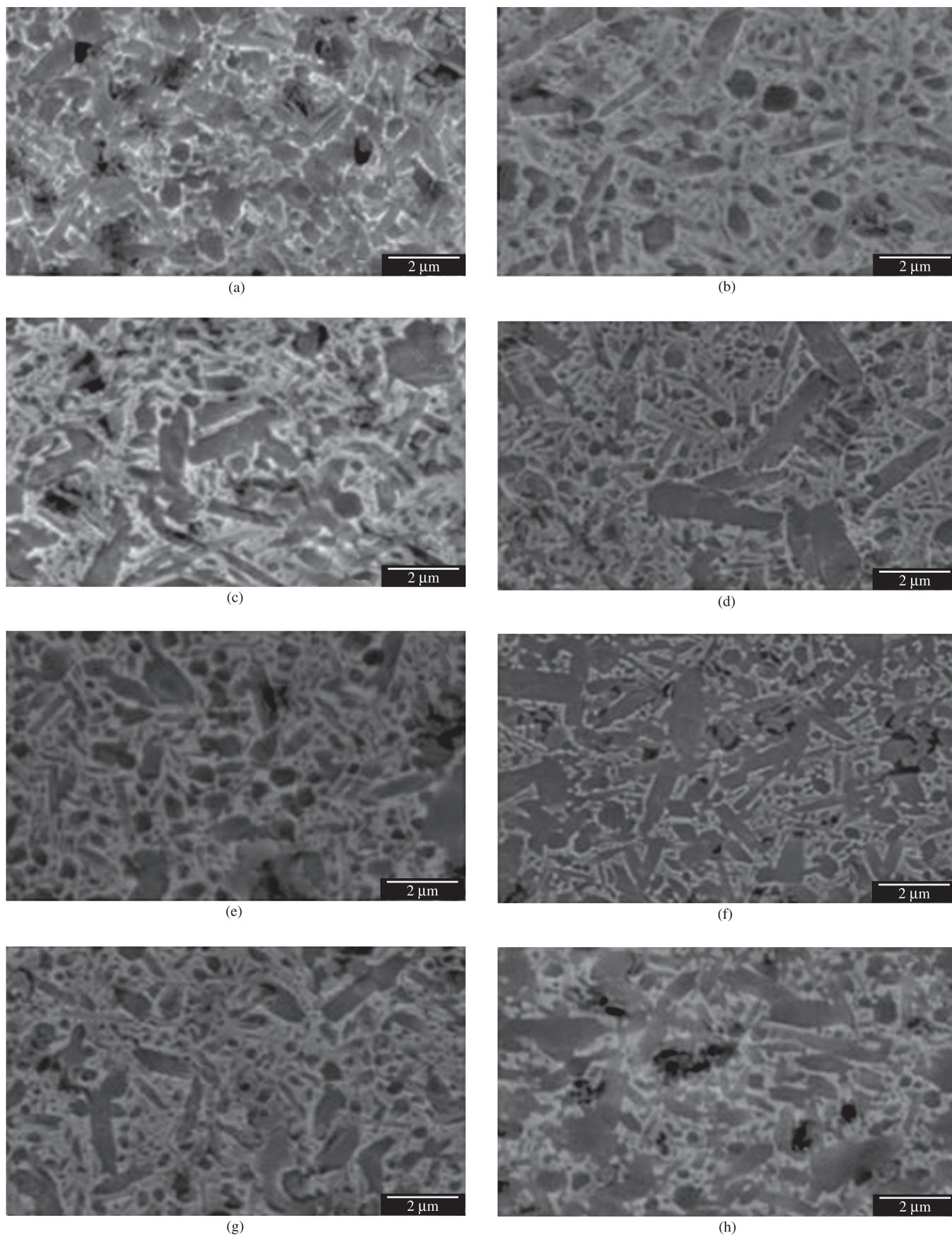
**Figure 2.** Scanning electron micrographs of plasma-etched silicon nitride-based ceramics with different additives (9 wt. (%)): a) SN-Y; b) SN-La; c) SN-Nd; d) SN-Dy; e) SN-Yb; f) SN-Y/La; g) SN-Y/Yb; and h) SN-Nd/Dy.
