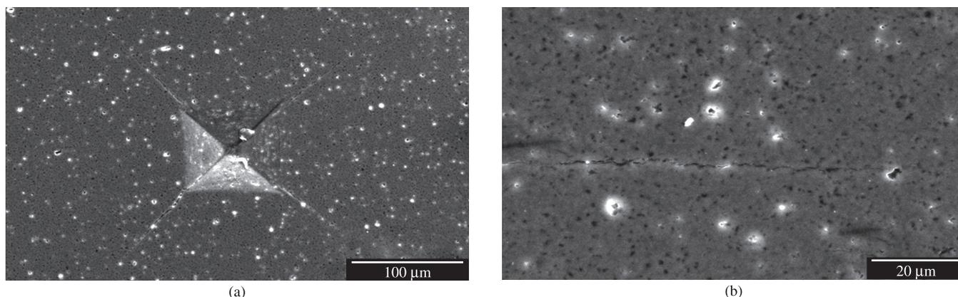
**Figure 3.** Typical scanning electron micrographs of: (a) Vickers indent; (b) propagating crack in silicon nitride based ceramics.
