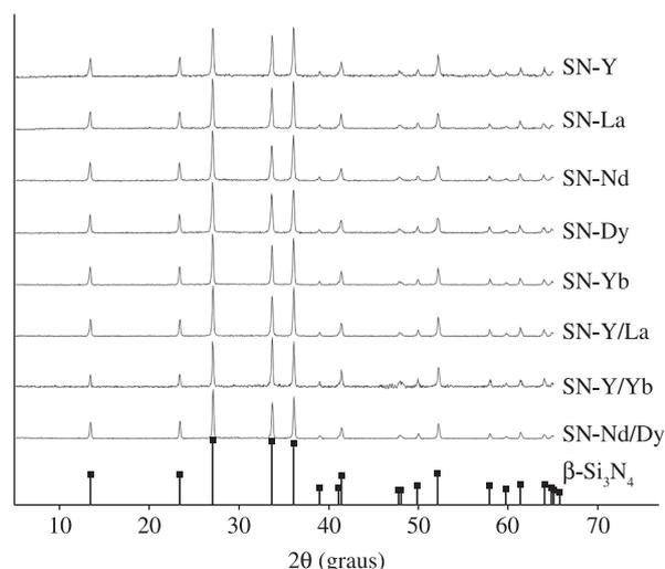
**Figure 1.** X ray diffraction (XRD) spectra of the silicon nitride samples.
