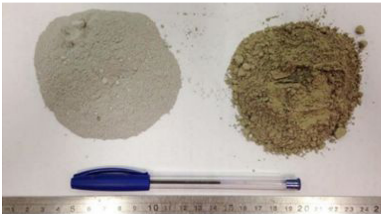
Figure 5. Visual comparison between silica fume (left) and cement (right), used in this research as binders.
