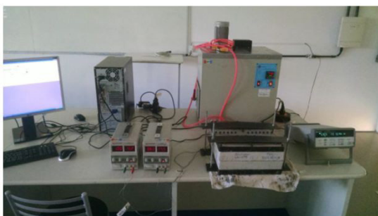
Figure 2. Bench for measuring thermal conductivity (a) and mounting the samples between the plates (b).
