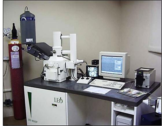
Figure 5. Scanning electron microscope LEO ZEISS model 1450 VP with Oxford Inca Energy spectrometer.
