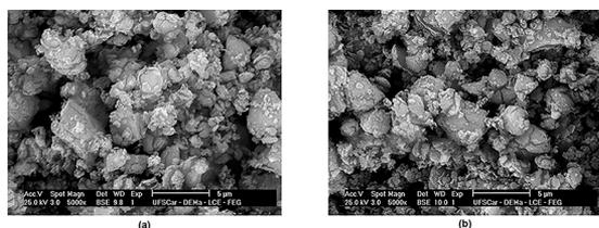
**Figure 4.** SEM micrographs (BSE images) for the nanocomposites: (a)  $\text{MgH}_2 + 5 \text{ mol\% TiCrV}$  and (b)  $\text{MgH}_2 + 5 \text{ mol\% TiCr}_{1.2}\text{V}_{0.8}$ .
