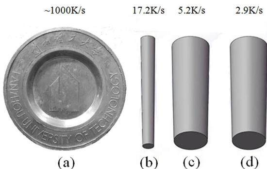
Figure 3. Schematic diagram of different forming mould (a) rheo-diecasting with thickness of 2mm; (b) permanent mould casting with diameter of 15mm; (c) permanent mould casting with diameter of 50mm; (d) sand mould casting with diameter of 50mm.
