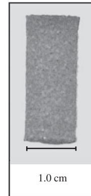
Figure 1. As sintered type 3 porous system, compacted at 200 MPa.
