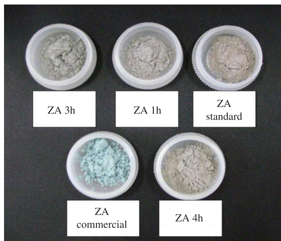
Figure 5. Images of pigments synthesized from zeolite A.
