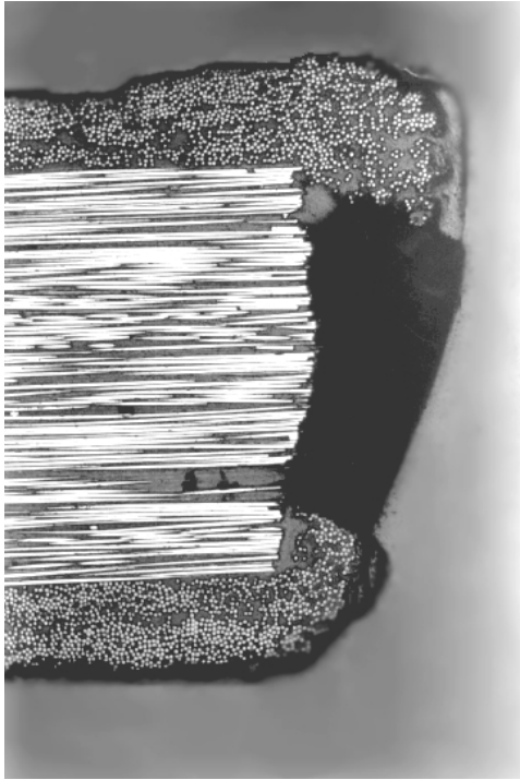
Figure 7. Micrograph of the cross section of a [0/90/90] s laminate with molded edge (100 X).
