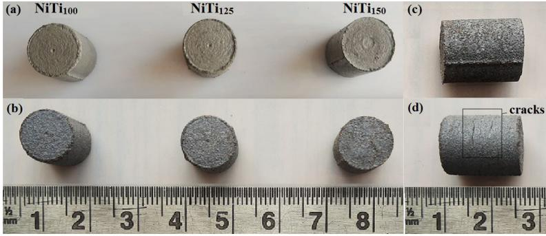
**Figure 4.** (a) NiTi composite samples after compaction at 1273.88, 1592.35 and 1910.82 MPa compaction pressure with sample id NiTi<sub>100</sub>, NiTi<sub>125</sub> and NiTi<sub>150</sub> respectively, (b) NiTi composite samples after sintering, (c) composite sample developed with ejector has no cracks on its circumference and (d) composite sample developed without ejector shows several cracks.
