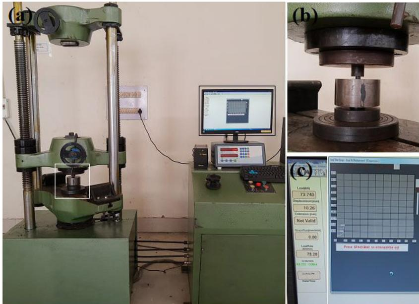
**Figure 2.** (a) Uni-axial compaction of NiTi composite powder on UTM, (b) enlarged view of white square showing die arrangement and (c) enlarged view of black square showing displacement of punch with UTM load.
