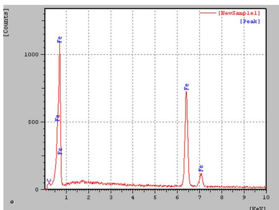
Figure 13. EDS analysis of uncoated diamond in point 03 of Figure 10.
