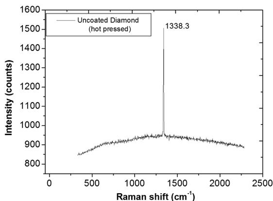
Figure 5. Raman spectroscopy of uncoated diamond, after hot pressing and chemical etching.
