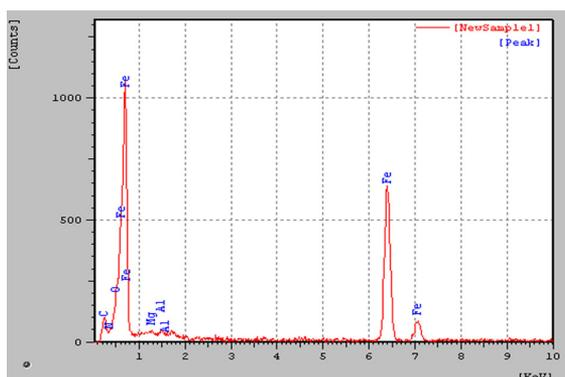
Figure 16. EDS analysis of TiC coated diamond in point 01 of Figure 15.
