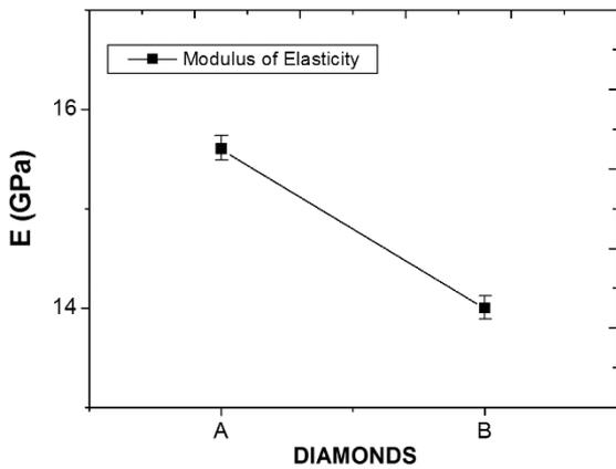
**Figure 8.** Modulus of Elasticity of diamond composites. A: uncoated diamonds composites and B: TiC coated diamonds composites.
