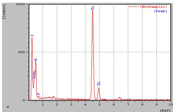
**Figure 18.** EDS analysis of TiC coated diamond in point 03 of Figure 15.
