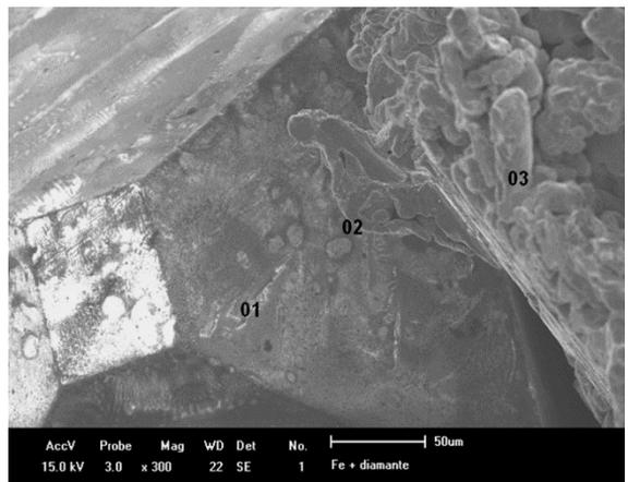
**Figure 10.** Micrograph of Fe-uncoated diamond composite after compression test. Points 1 to 3 are regarded to EDS analyses.
