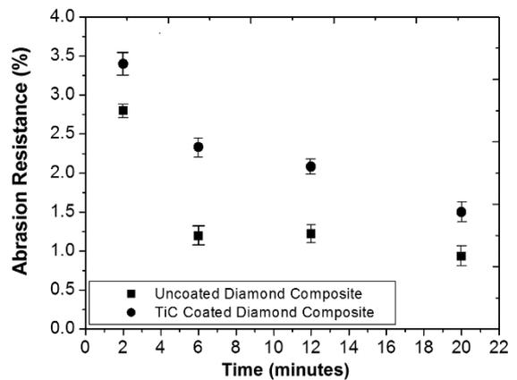
**Figure 19.** Abrasion Resistance (AR %) of Fe-diamond composites as a function of time. Mean values for three samples of each system.
