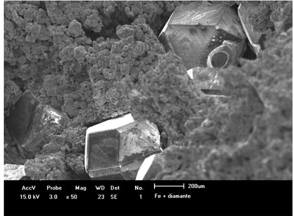
**Figure 9.** Micrograph of uncoated Fe-diamond composite after compression test.
