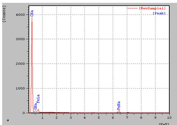
Figure 12. EDS analysis of uncoated diamond in point 02 of Figure 10.
