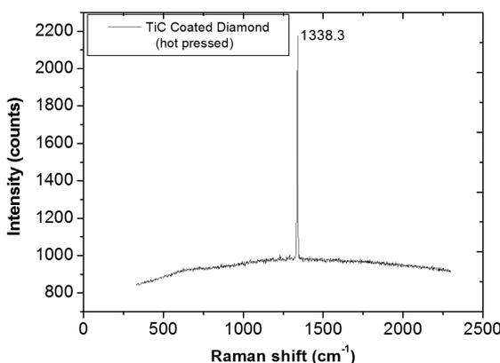
Figure 6. Raman spectroscopy of TiC coated diamond, after hot pressing and chemical etching.
