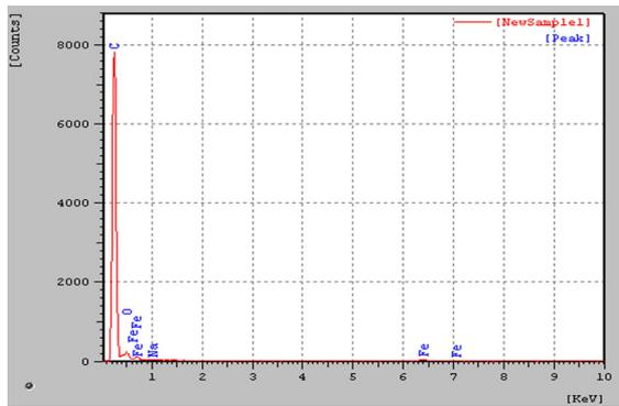
**Figure 17.** EDS analysis of TiC coated diamond in point 02 of Figure 15.
