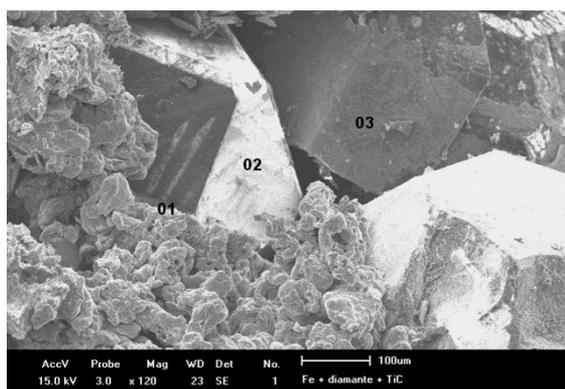
Figure 15. Micrograph of Fe-TiC coated diamond composite after compression tests. Points 1 to 3 are regarded to EDS analyses.
