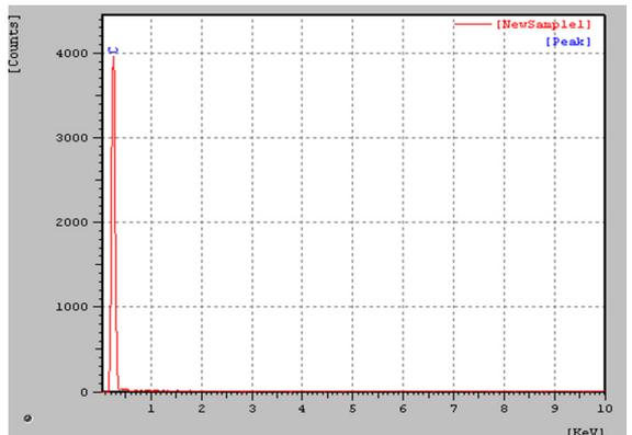
**Figure 11.** EDS analysis of uncoated diamond in point 01 of Figure 10.
