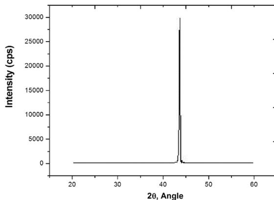
Figure 1. XRD pattern. Diamond crystals as received from the manufacturer.
