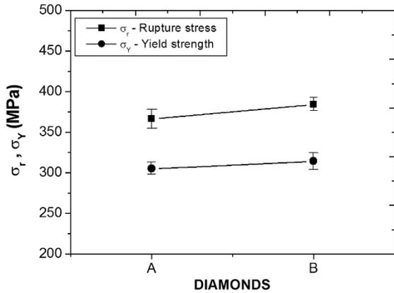
**Figure 7.** Rupture stress ( $\sigma_r$ ) and yield strength ( $\sigma_y$ ) of diamond composites. A: uncoated diamonds composites and B: TiC coated diamonds composites.
