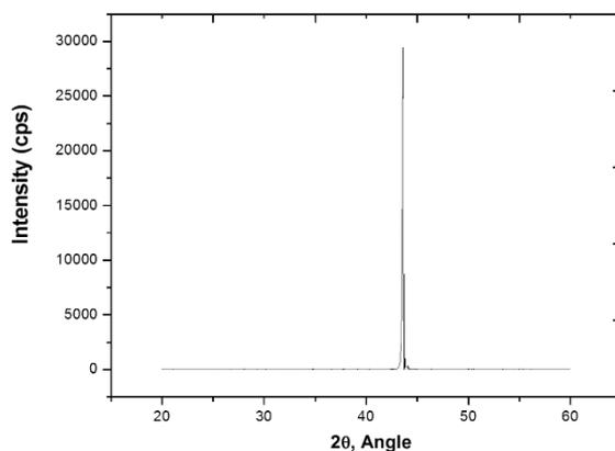
Figure 2. XRD pattern. Uncoated diamond crystals (hot pressed).
