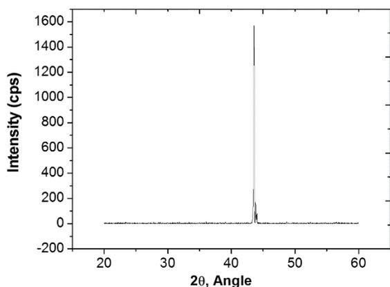
Figure 3. XRD pattern. TiC coated diamond crystals (hot pressed).
