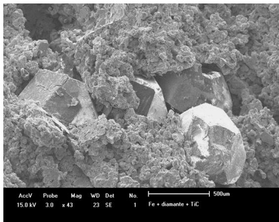
Figure 14. Micrograph of Fe-TiC coated diamond composite after compression tests.
