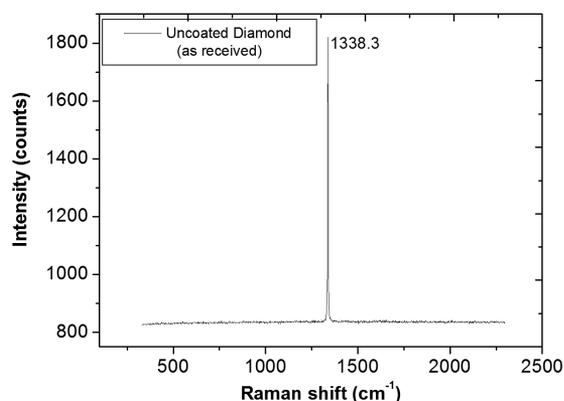
Figure 4. Raman spectroscopy of diamond crystals as received from the manufacturer.
