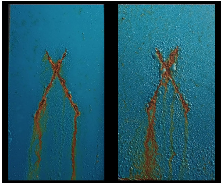
Figure 11. Coating after 300 hours salt spray exposure (ASTM B117 75 ) Strong osmotic blistering due to water soluble contaminant in graphene dispersion. Right: no graphene. Left: graphene.
