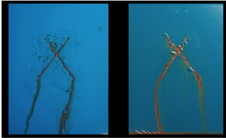
Figure 10. Coating without anodic protection technology after 300 hours salt spray exposure (ASTM B117 75 ): increase of corrosion product due to galvanic corrosion between graphene and steel substrate. Left: no graphene. Right: Graphene.
