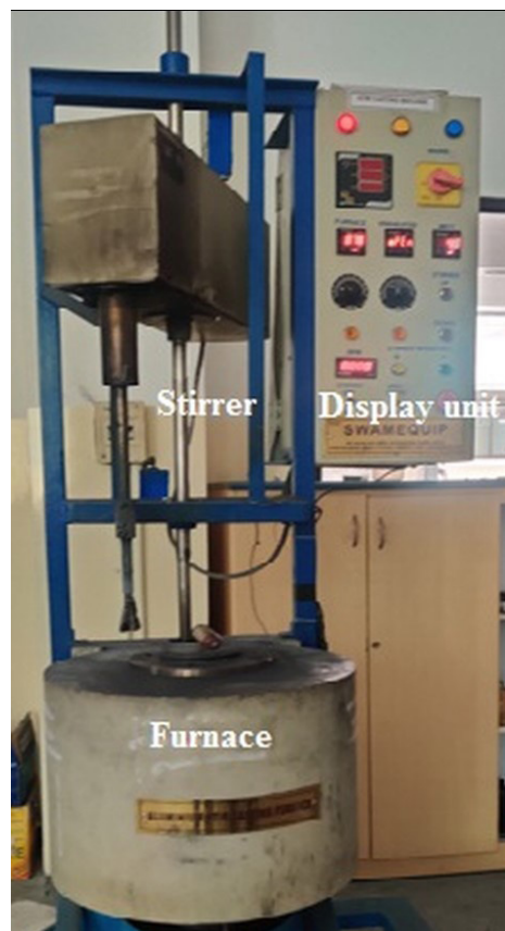
Figure 2. Stir casting equipment used in this investigation.
