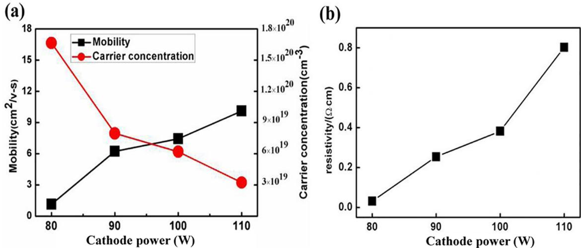
**Figure 5.** (a) Hall mobilities and carrier concentrations of InN samples deposited on sapphire substrates at different sputtering powers, (b) Resistivities of InN samples at different sputtering powers.
