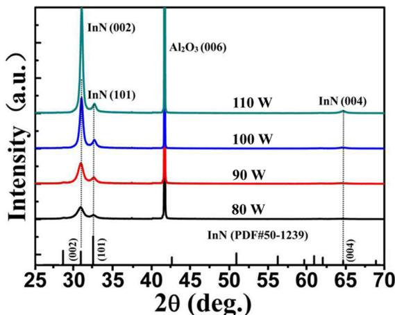
**Figure 1.** w-2θ XRD scans of InN samples deposited on sapphire substrates at different sputtering powers.
