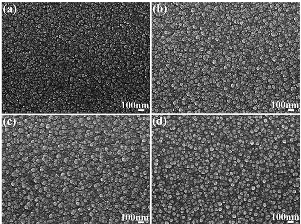
**Figure 3.** SEM images of the InN samples grown at different sputtering powers: (a) 80W, (b) 90W, (c) 100W and (d) 110 W.
