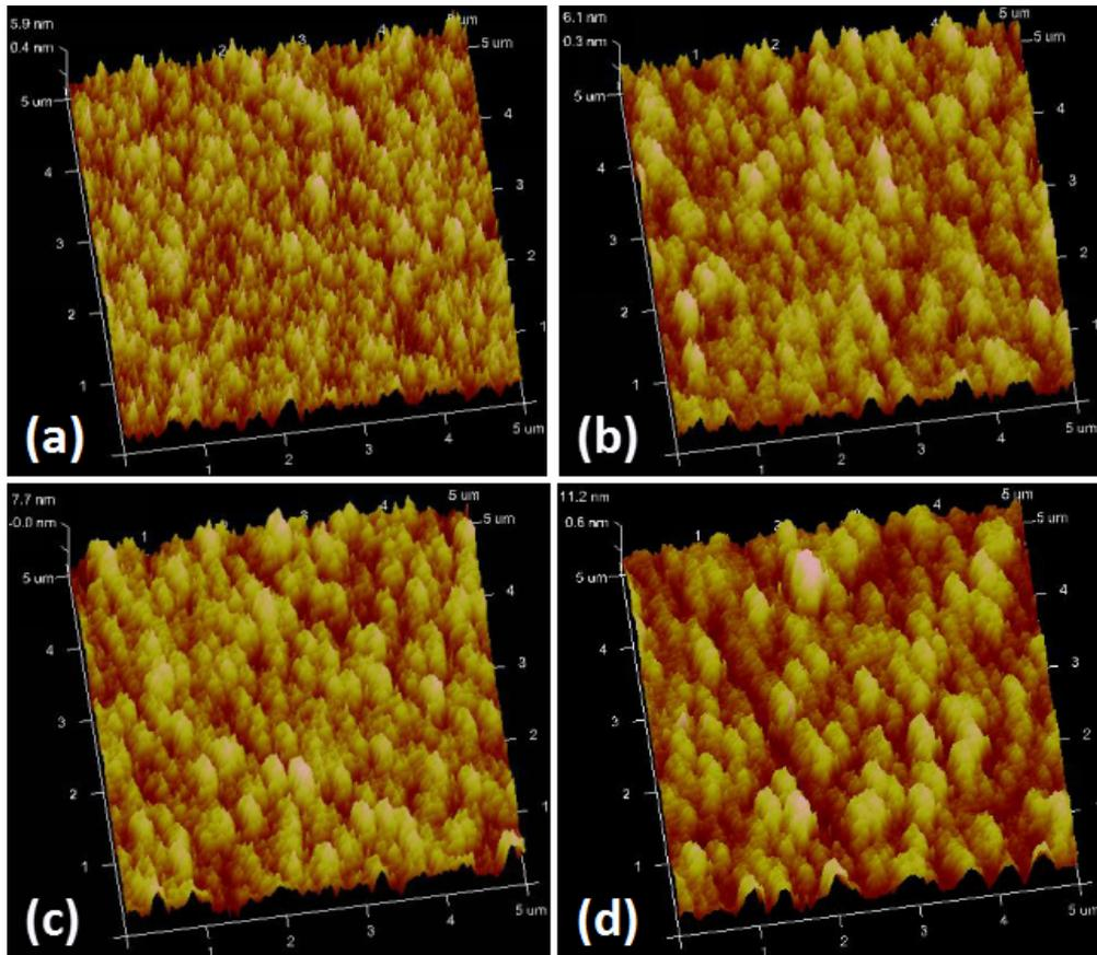
**Figure 2.** 3D morphology of the AFM images ( $5 \times 5 \mu\text{m}^2$ ) of the InN nanodots grown at different sputtering powers: (a) 80W, (b) 90W, (c) 100W and (d) 110 W.
