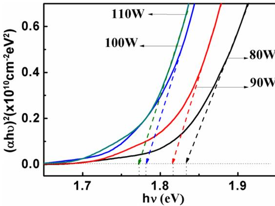
**Figure 4.** Optical absorption spectra of InN samples deposited on sapphire substrates at different sputtering power: 80 W, 90 W, 100 W and 100 W.
