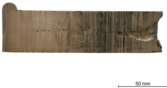
Figure 1. Typical example of cavities at a large volume casting sample of P1
