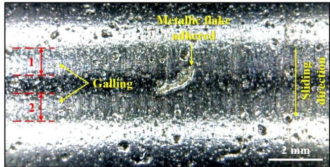
**Figure 14.** (a) Schematic representation of acting forces in the formability tests and contact pressure distribution (region AB) on the bending pin surface and (b) Appearance final of the pin surface after severe wear. Reference: Paper authors. Analysis performed during this research.
