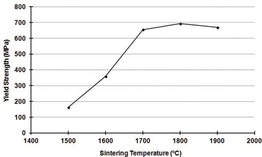
**Figure 5:** Yield Strength as a function of sintering temperature.
