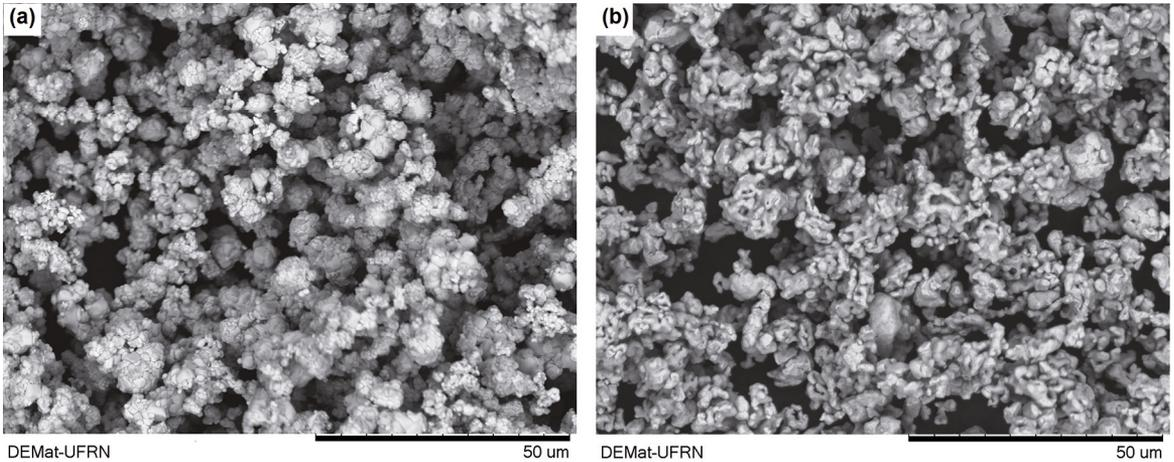
**Figure 1:** SEM morphologies of as-received powders. (a) WC and (b) Co.
