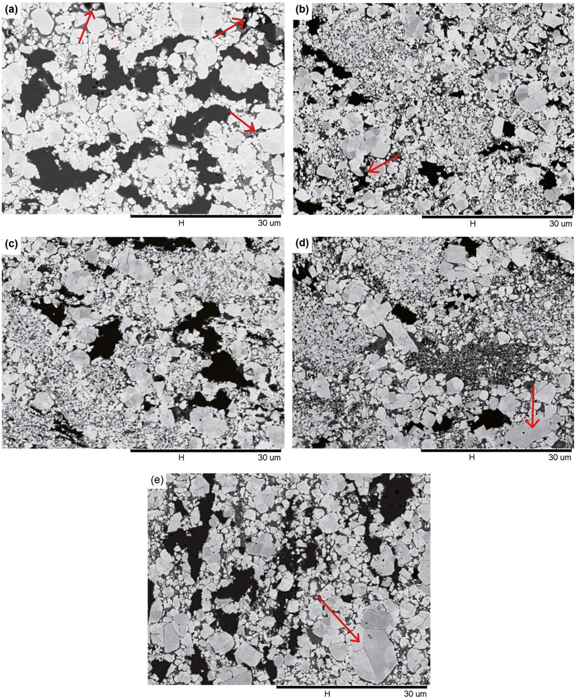
**Figure 3:** SEM metallographic images of sintered WC-10Co at different temperature. 1500°C (a), 1600°C (b), 1700°C (c), 1800°C (d), and 1900 °C (e). Porosity in lower temperature and abnormal grain growth in higher temperature.
