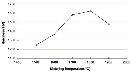
**Figure 4:** Vickers hardness as a function of sintering temperature.
