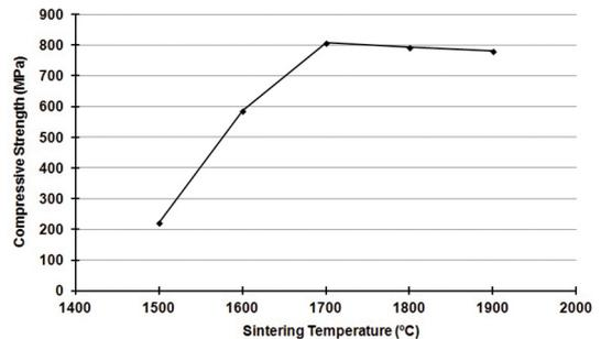
**Figure 6:** Compressive strength as a function of sintering temperature.
