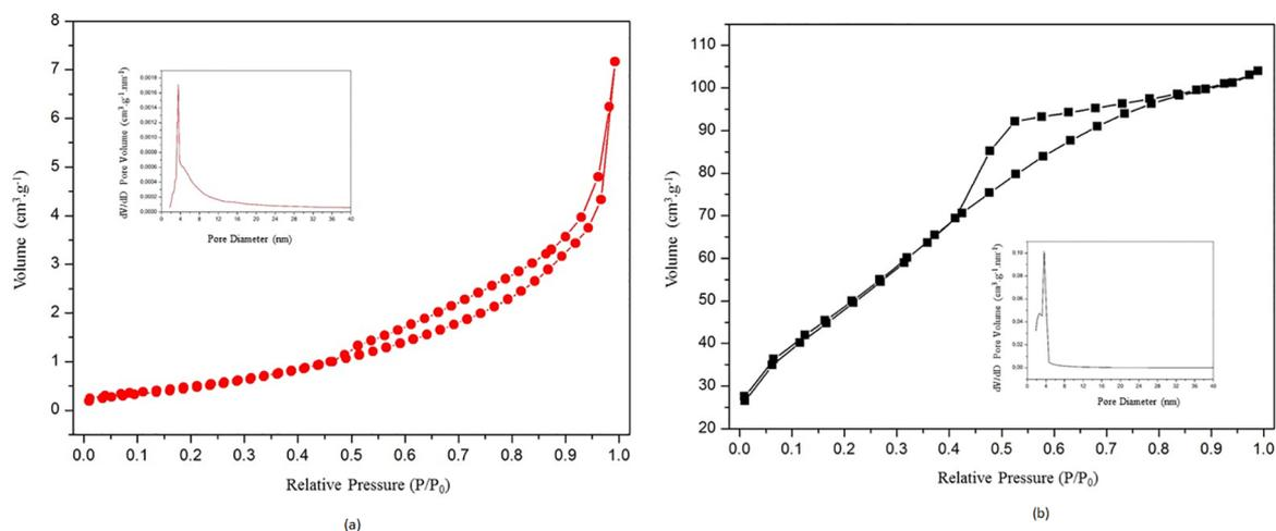
**Figure 3.**  $N_2$  adsorption/desorption isotherms and (insert) pore diameter distribution of (a)  $ZnAl_2O_4\_MC$  and (b)  $ZnAl_2O_4\_H$  powders.
