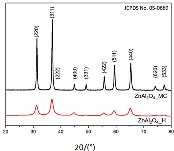
**Figure 1.** XRD patterns of ZnAl<sub>2</sub>O<sub>4</sub> powders.
