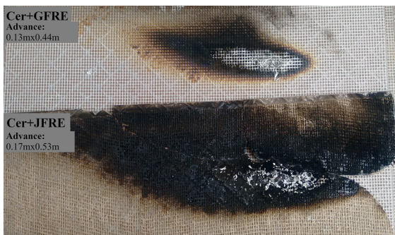
Figure 10. Comparison of the conjoint composites after the flame propagation test.
