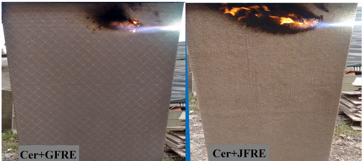
Figure 9. Initial moments in the flame propagation test.
