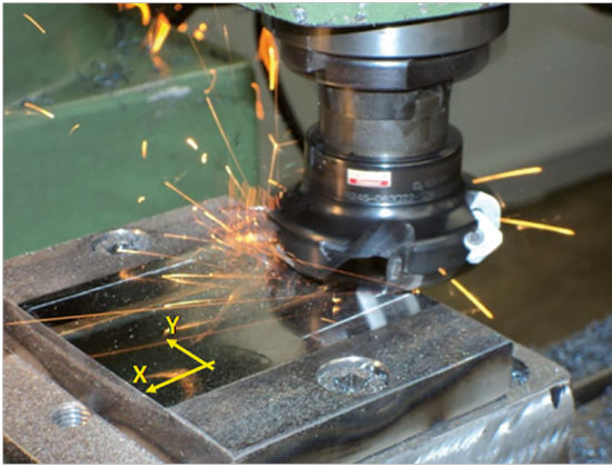
Figure 1. Setup assembly showing the axes configuration used for the residual stresses tests.
