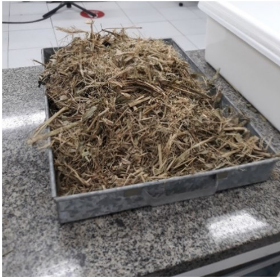
Figure 1. Bamboo fibers after drying in an oven.
