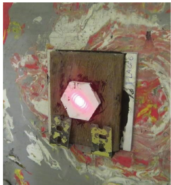
Figure 4. Actual view of a clamped MAS with giant bamboo composite plate ready to be ballistic tested. Laser beam focusing in the center of the ceramic plate as sight. Source: authors.
